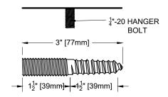
2.2 IDENTIFY THE THREADED END OF THE BARREL AND THE SWAGE END OF THE CABLE. INSERT THE PLAIN WND OF THE SUPPLIED WIRETHROUGH THE LARGE THREADED END OF THE BARREL UNTIL IT IS FULLY SEATED IN THE BARREL. ATTACH THE THREADED END OF THE BARREL TO THE 1/4"-20 HANGER BOLT.
