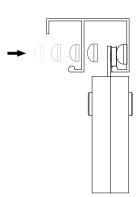
b. Attach Rubber bump stops at the end of aluminum channel.
