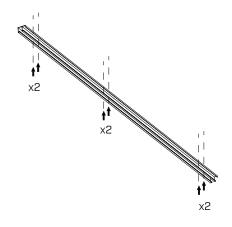
**a.** Drill 6 holes spaced as above.
