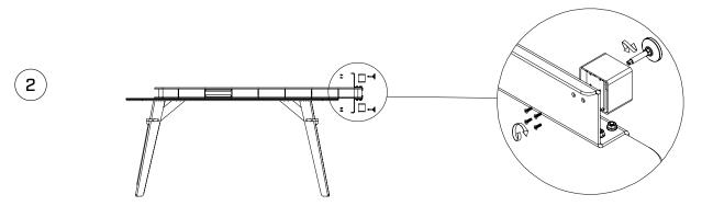
Insert countersunk bolts, adjustable feet housing and then tighten bolts with right sizes Allen Key. Repeat for all bolts
