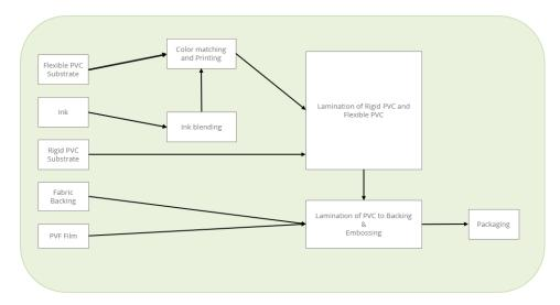
Figure 1. Manufacturing diagram for P3TEC Advanced Wall Protection.
