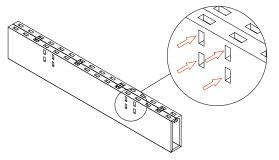
2.2 FOR INSIDE BEAMS REMOVE PRE-CUT RECTANGULAR HOLES ON BOTH SIDES.
