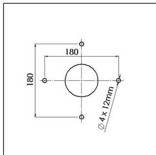
Because of the flat bottom and bolt guides, there are many ways to attach the pump. For example, this may be installed on a concrete flagstone, by setting it into a foundation or anchoring it in composite stone. Fixing material included in delivery: 4x plastic wall plugs 12mm and 4x screws
