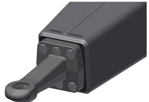
**Drawbar with ASP and trailer ring with flange**
