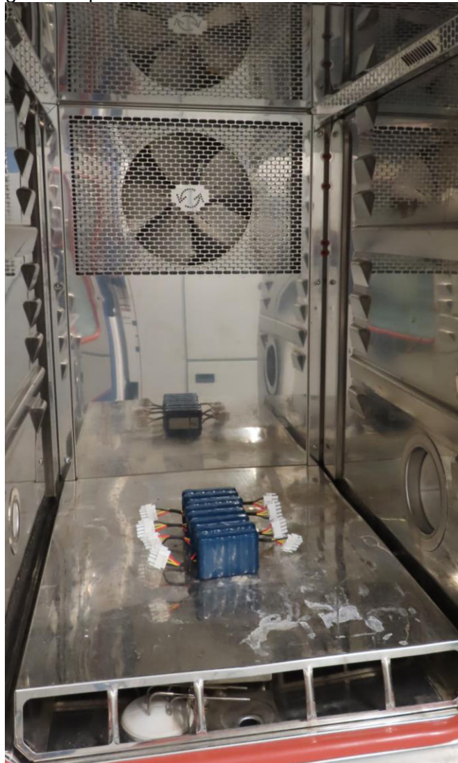
Figure 7: Specimen inside of the climatic test chamber
