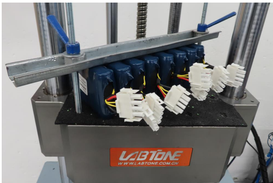
Figure 17: Specimens fitted toward -Y direction (the test is conducted by parts, the minus direction obtained by turning the sample)
