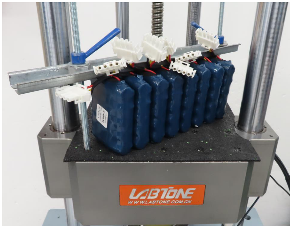
Figure 18: Specimens fitted towards Z direction
