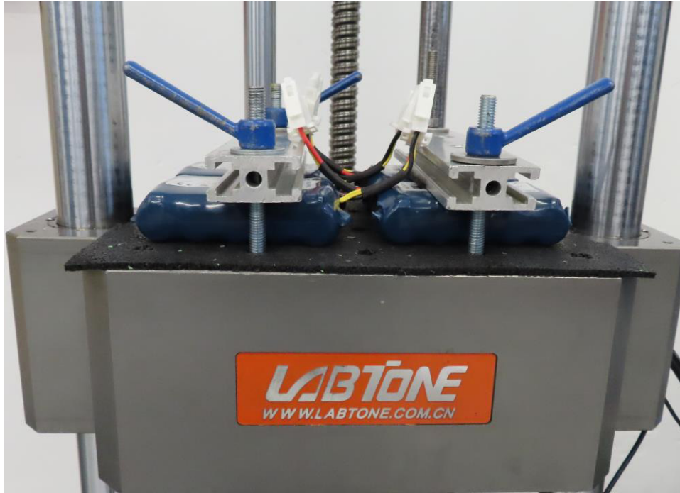
Figure 17: Specimens fitted toward -Y direction (the test is conducted by parts, the minus direction obtained by turning the sample)
