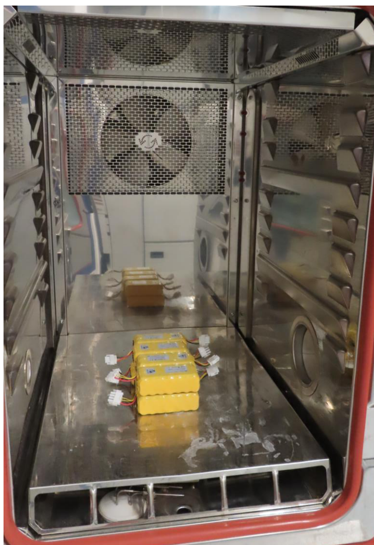
Figure 7: Specimen inside of the climatic test chamber
