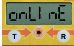
This function is used to enable or disable modem communication. **IMPORTANT:** If the modem is offline, alarms are stored in the system memory but are not automatically saved because they are not sent to the server.
