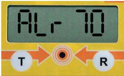
This function is used to set the default value for the alarm message "too hot" (default setting 70°C)
