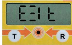
This function allows you to exit master mode and initiates a display reset.
