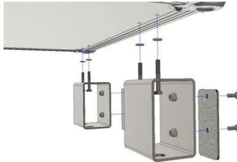
5. Secure the fastening screws using washers and hexagonal nuts on the inside of the cabinet.
