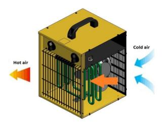
The device works on the principle offorced convection . The air flow is forced fan. Cold air is drawn in the back of the unit. Further washes flowing from the heater receives heat. The heated air is expelled in front of the heater. The device has a thermostat for the regulation temperatures 5-35  $^{\circ}$ C. The unit area equipped with thermal protection is acting automatically. The unit features: ventilation, heating with half the power, heating at full power.
