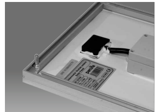
Insert two screws (M6x16) each at the top and on the bottom of the aluminium frame of the solar panel.
