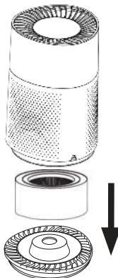
3. The filter and housing base can now be removed downwards.
