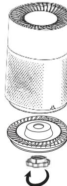
2. Unscrew the large twist lock on the underside.
