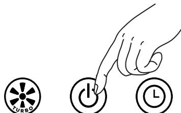
6. Press and hold the ON/OFF button on the activated air filter for 20 seconds until the red FILTER indicator goes out.
