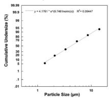
Measurements were performed using a sodium fluoride solution with a "Next Generation Impactor" (NGI).
