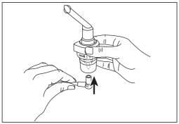
Connect the other end of the compressed air hose [8] to the nebuliser hose connection [6] by turning it slightly.
