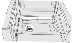
4.) Insert the plug attached to a spiral spring into the socket provided. Then fold the seat cushion against the back rest.
