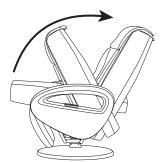
3.) Unfold the back rest to the upright position until the locking mechanism audibly engages.
