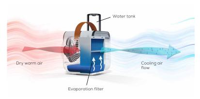
The air fan draws in the dry warm air from the room, which then comes into contact with the evaporation filter, which is saturated with water. The contact between the air flow and the damp filter surface causes the water to evaporate. The ambient air absorbs the humidity, and the thermal energy required for the evaporation process is extracted from the ambient air. There is a noticeable drop in the temperature of the ambient air.
