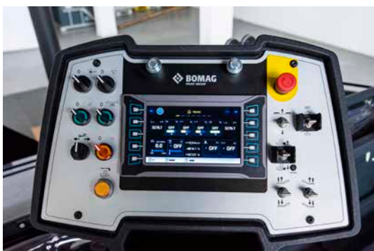
The new control centre. The intuitive operator interface not only provides all the necessary information, but also supports the operator with assistance functions.
