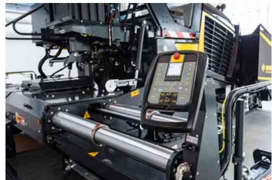
Full control from the side. The integrated levelling controller and automatic inclination ensure perfect quality.
