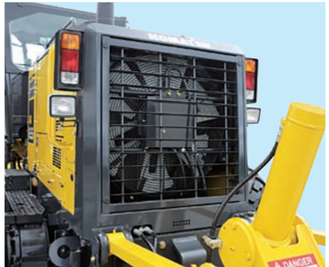
Hydraulic driven cooling fan
