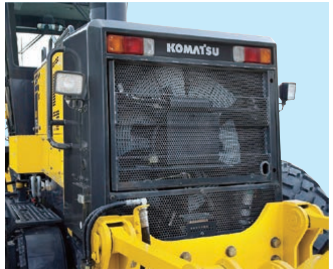
Hydraulic driven cooling fan
