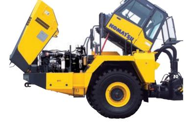
The number of grease points are minimized by using maintenance-free rubber bushings.
