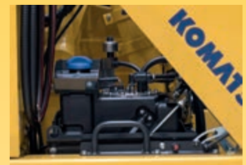
Simple access to the AdBlue® tank
