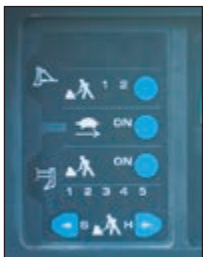
Track shoe slip control panel
