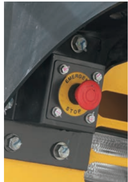
Three emergency engine stop switches are installed in the cab and around the machine.
