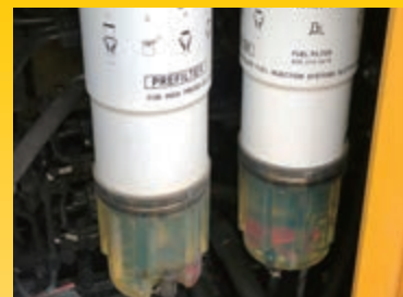
Large capacity fuel pre-filter with water separator
