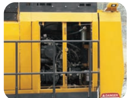
Bulkhead wall (fire wall) prevents oil from splashing into the engine room in the event of hydraulic oil leak.
