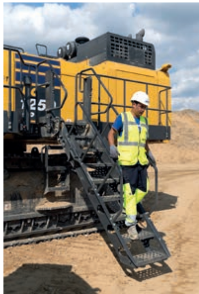
The hydraulically operated stairway provides safer access and egress to and from the machine.
