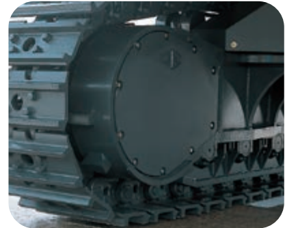
Sturdy travel motor guards and rock protectors
