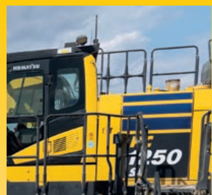
Hand rails and anti-slip plates
