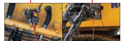
Emergency engine stop switch (optional)
