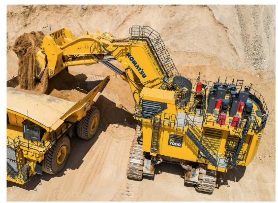
Keep your trucks productive with the intelligent, robust and versatile PC7000. Its 38m<sup>3</sup> shovel is sized to cycle big loads fast, while its advanced intelligent data solutions and performance monitoring can help you optimize the transfer of every load.
