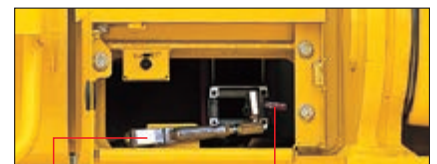
Grease gun The grease gun can be reached from ground level.
