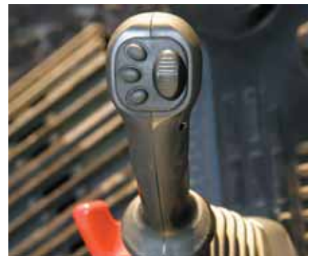
Joysticks with proportional control button for attachments
