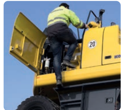
Handrails and anti-slip plates
