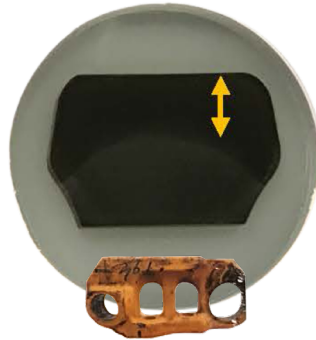
Link portion heat treatment has a larger depth on Komatsu link part. (Higher hardened depth, yellow arrow).
