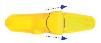
New tooth and wear cap redesigned to deflect material flow away from the adapter improving the assemblage's overall wear life.
