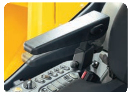
Armrest with simple height adjustment
