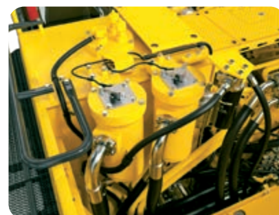
Return oil filter clog detection function recommends filter exchange and prevents catastrophic damage of hydraulic system.
