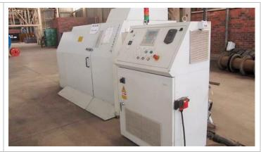
2012 SAMP 1250 Double 10 Twist Buncher and Lay-up Machine Including: 5 x SAMP SV1250DMN-P Pay-off Stations Serial number: 2012T01902 Serial number: 2012T01903 Serial number: 2012T01904 Serial number: 2012T01905 Serial number: 2012T01906 Including SAMP APC3 Control Serial number: 2012T01901 Including Siemens Electric / Electronic Switchgear with Siemens drives and Control Panel, Piping, Cable and Foundation
