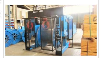
13 2013 SKALTEK MP400 Coiling Machine Including: Skaltek AX20-2 Pay-Off with Control Serial number ZA1105-2786-10 Skaltek MP400 Pure Coil Packer Serial number: ZA1105-2786-20 Skaltek SW4 & S04 Shrinkwrapper Serial number: ZA1105-2786-30 Skaltek S04 Drying Tunnel Including Siemens Electric/Electronic Switchgear with Siemens drives and Control Panel, Piping, Cable and Foundation
