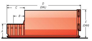
Dimensions not shown: 8'41/8" (2543mm) Overall Width Ground Roller Widths: 61<sup>7</sup>/<sub>8</sub>" (1569mm) Inside Rollers
