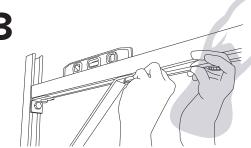
Make sure the horizontal Slotted Track is level. Adjust if necessary. Mount the remaining 24" Slotted Tracks horizontally and protruding from the wall so that the slotted surface of the Slotted Track is 4.25" below the top edge of the vertical 24" Slotted Track. Use the Knee Braces, Angle Brackets, and the Spring-loaded Nuts and Hex Head Cap Screws to secure the horizontal Slotted Track in place.
