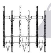
Secure the DUPLEX ASSMBLY with 3/8" WEDGE ANCHORS. Secure at the first and last pair of bases and then every other pair of bases.
