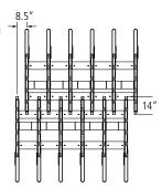
For double sided assemblies, simply place two single sided assemblies back to back with a 14" overlap.
