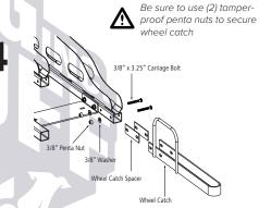
Place WHEEL CATCH and SPACERS and attach with hardware. Repeat for all trays.
