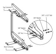
Place the first DUPLEX LOWER UNIT and attach CONNECTORS with hardware.
