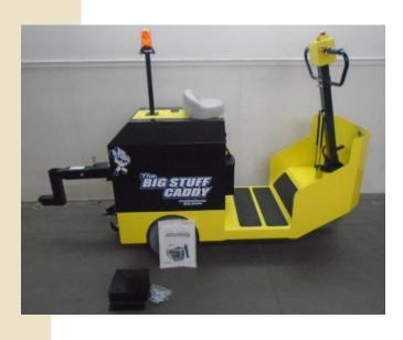
Used for moving sausage bag compactor trash or collecting general debris. Multiple options for tip bin size and height. Models range from 1,000lb capacity to 5,000lbs capacity over a flat surface. Slight to steep inclines.
