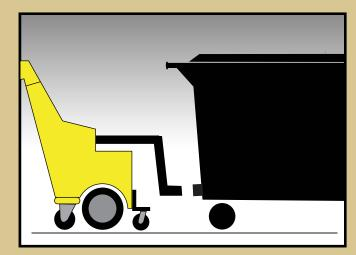
Insert tube on the front of the Big Stuff Caddy attaches to the bottom of the dumpster.
