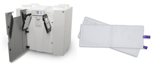
The filters are situated behind the door of the MVHR unit. Press the filter symbol for longer than 3 seconds to open the filter wizard. Follow the instructions that appear on the display to clean or replace the filter. If the filters are not particularly dirty, they can be vacuumed and cleaned using a detergent and gently washed under running water. Leave to air dry before returning them to the MVHR unit.
