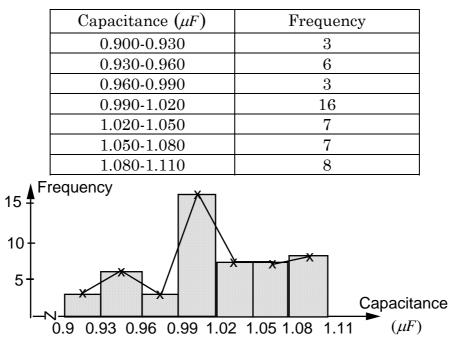
Histogram and frequency polygon showing the capacitance measurements of  $1\mu F$ .
