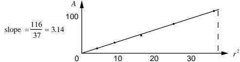
The intercept = 0 and gradient = 3.14. So k = 3.14 and b = 0. The results in the table seem to be obtained from the formula for the area of a circle  $\pi r^2$ .
