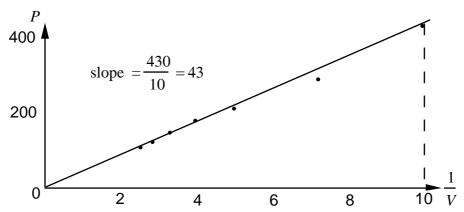
(iii) P against 1/V is a straight line through the origin, so the intercept is equal to zero, hence  $P = \frac{k}{V}$  where k is the gradient. Since k = 43 we have
