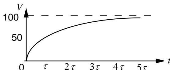
The percentage of  $V_0$  after  $t = \tau, 2\tau, 3\tau, 4\tau$  and  $5\tau$  is 63.2%, 86.5%, 95%, 98.2% and 99.3% respectively. [Note: The capacitor has a voltage  $V_0$  (approximately) after 5 time constants ( $5\tau$ )].
