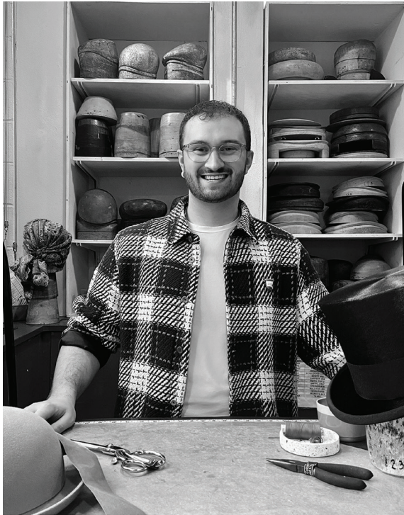
Figure E4.2 Tommy with his collection of hat blocks. Typically made of wood, they are used to mould the felt, straw and other millinery materials to form the desired shape. © Tommy Cobau
