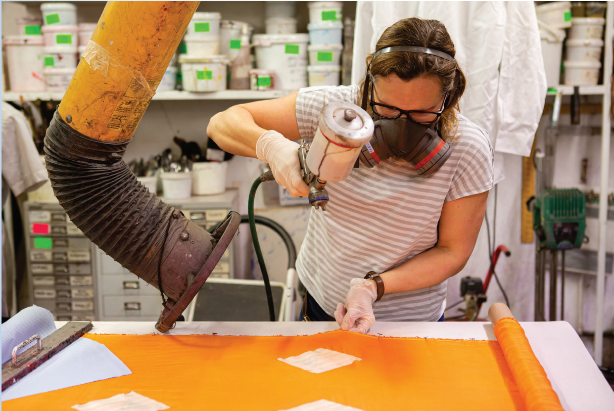
Figure E4.6 Protect those lungs! Spray-painting emits a fine mist which can be inhaled, so the appropriate mask must always be worn. © Nicola Killeen Textiles/Kevin Meredith
