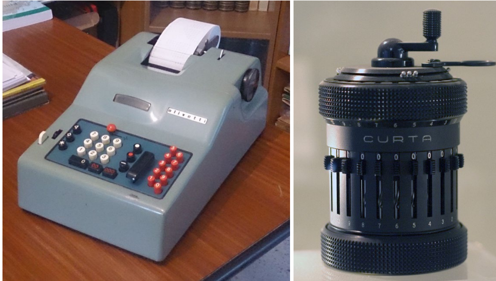
Fig. 9.1 - examples of mechanic calculator: on the left side (a) Olivetti Divisumma, 1947; on the right side (b) Curta portable calculator).
