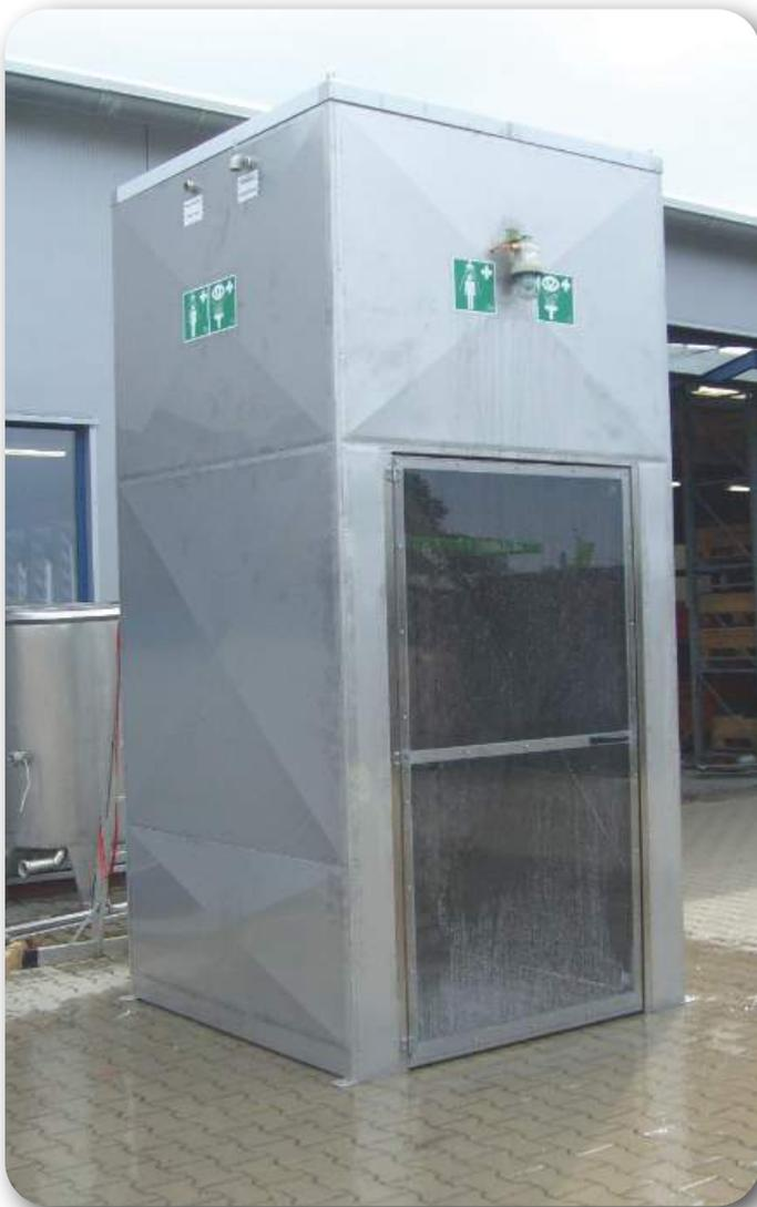
The basic design consists of a massive, stainless steel square-tube frame with top-mounted stainless steel tank including an airtight cover and statics quality inspection according to DIN EN 1055. The tank is insulated on all sides and jacketed with stainless steel panels. All tank safety showers are suitable for EX-zones 1 & 2. you have to mind, if the afterwards use is in EX-zones, before selection of the options.
