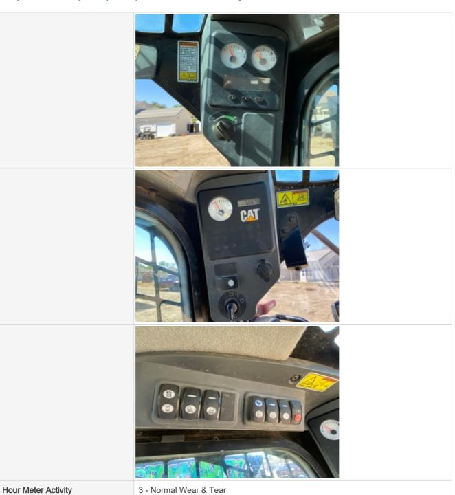
Hour meter is functional and in good condition
