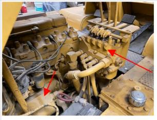
Arrows pointing at Hydraulic Pump (on the left) & Main Control Valve (on the right)
