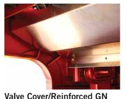
A protective panel on the underside of the gooseneck shields the hydraulic valving from road grime & debris. To prevent cracking and provide extra strength, the gooseneck is reinforced with a gusset and a brace
