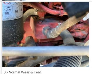
Overall drivetrain in solid shape. Minor leak at trans oil pan or around it observed. Additional Undercarriage Components
