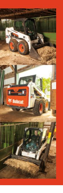
The skid-steer loader can pivot 360 degrees, which makes it one of the most maneuverable pieces of equipment available.
