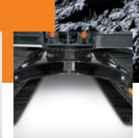
■ Thick-plate single-sheet mainframe, box-section track frames and industry exclusive double-seal swing bearing deliver rock-solid durability.
