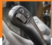
■ Ergonomically correct shortthrow pilot levers provide smooth, precise control with less effort. Pushbuttons in the right lever allow control of auxiliary hydraulic flow for attachments. Optional sliding switch provides proportional speed control, giving you full command from your fingertips.
