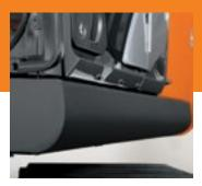
Reinforced D-channel side frames provide maximum cab and component impact protection.
